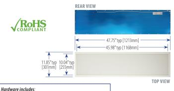
(1) Junction Box w/ Power Supply (L: 7.95 x W: 3.30 x H: 1.38) (2) White Aluminum Rails (L: 47-3/4 x W: 1.38 x H: 0.77) Junction
